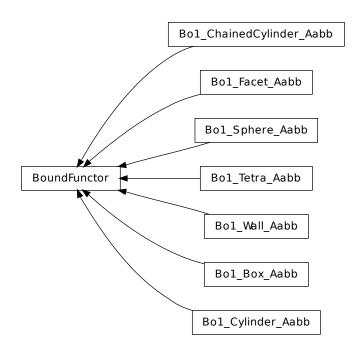
${\tt class \ yade.wrapper.BoundFunctor}(inherits \ Functor \rightarrow Serializable)$
