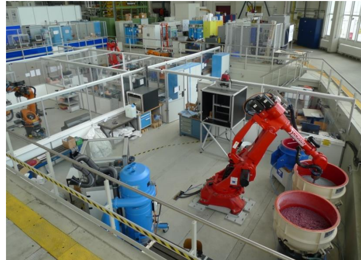
Robot Cell for Finishing Operations at IWF, TU Berlin
