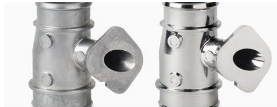
Fitting before and after vibratory finishing [Walther Trowal GmbH & Co. KG ]
