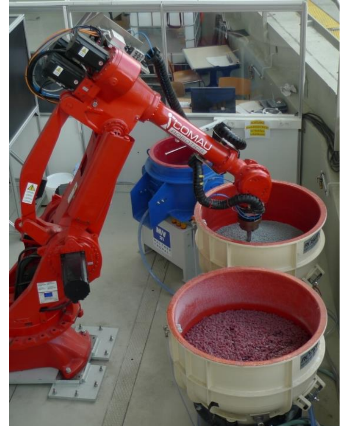
Robot guided drag finishing and vibratory finishing facilities at IWF, TU Berlin
