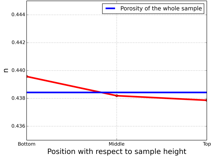
Figure 9: Local porosities at different sections of the eroded sample under a hydraulic gradient, i = 3 .
