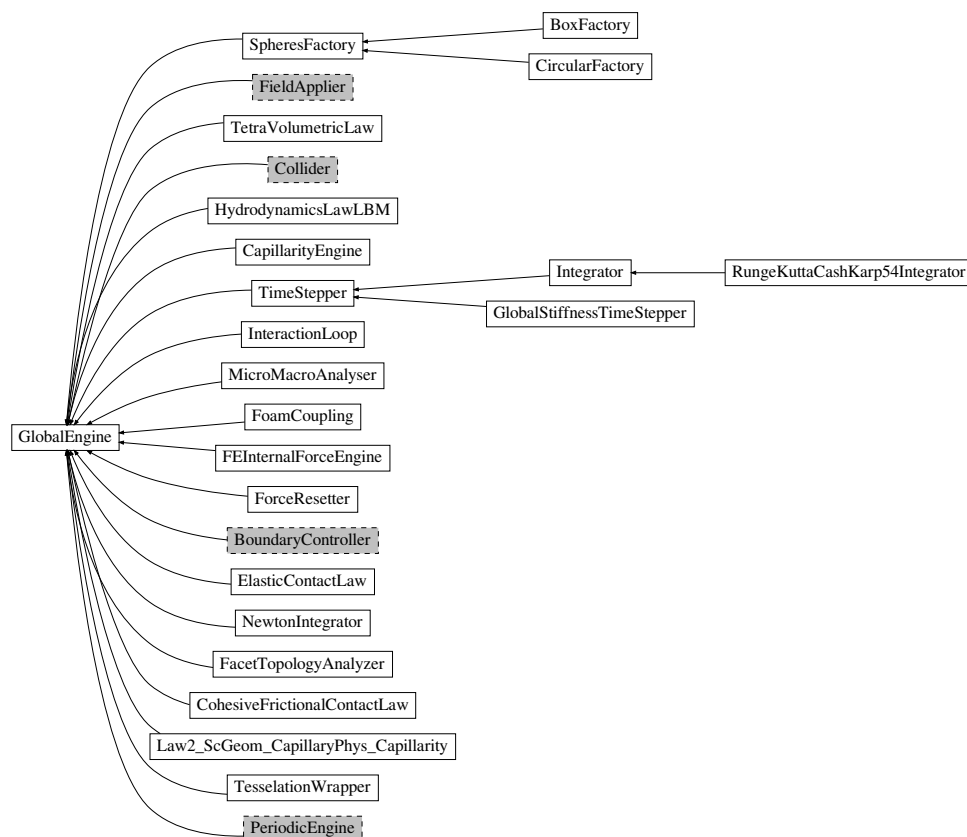
Fig. 25: Inheritance graph of GlobalEngine, gray dashed classes are discussed in their own sections: FieldApplier , Collider , BoundaryController , PeriodicEngine . See also: BoxFactory , CapillarityEngine , CircularFactory , CohesiveFrictionalContactLaw , ElasticContactLaw , FEInternalForceEngine , FacetTopologyAnalyzer , FoamCoupling , ForceResetter , GlobalStiffnessTimeStepper , HydrodynamicsLawLBM , Integrator , InteractionLoop , Law2_ScGeom_CapillaryPhys_Capillarity , MicroMacroAnalyser , NewtonIntegrator , RungeKuttaCashKarp54Integrator , SpheresFactory , TessellationWrapper , TetraVolumetricLaw , TimeStepper .
